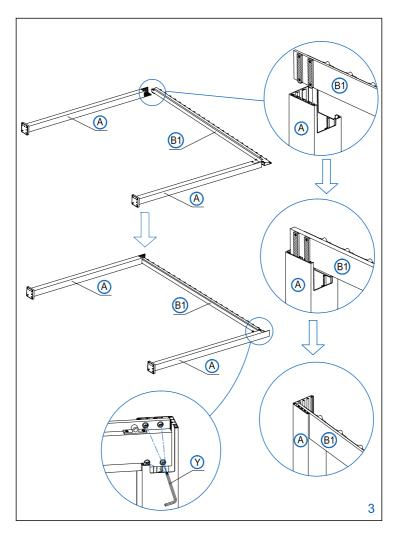
Lay down the other two leg sections (A) on the ground as shown. Take the (B2) rail and slide each end into position in the grooves along the top of the leg sections, just like the previous step. Use large allen key (Y) to affix the four screws on each corner.
