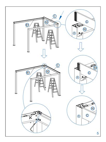
Move the ladders to the other side of the structure. Install the other beam (C) onto the open end, using the same method as in Step 5.
