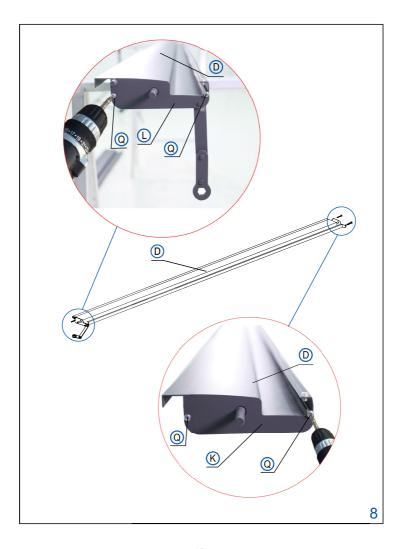
Move this louvre to the top of the structure, lining up the louvre arm (L) with the crank socket on the B1 rail, just above the crank handle. Insert the crank bolt of the louvre arm into the crank socket. Insert the pin on this end of the louvre into the second hole position on top of the B1 rail. Place the pin on the other end of the louvre in the second slot position on top of the B2 rail.
