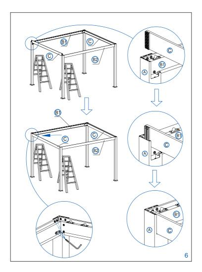
Find the corner below along the B1 rail with the crank pin hanging down. Remove the screw from the crank pin temporarily. Slide the crank loop (V) over the pin, lining up the holes. Drive the screw through both parts. Insert the hook of the crank handle (H) through the crank loop (V).
