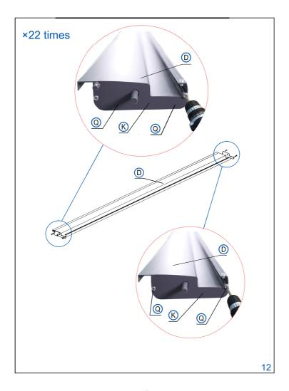
Install one of these louvres into the first position, next to the beam. Ensuring this louvre is in the same orientation as the one already installed, insert the pin on the crank handle end into the first hole position on the B1 rail. Place the pin on the other end of the louvre into the first position slot. Place a small cover (M) on top and screw down in place using two M5 screws (P).
