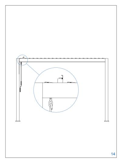
Once all louvres are correctly installed, take the louvre guide rail (G) and line up the holes with the free louvre pins on the crank handle side. Put the louvre guide rail over the pins as shown below. Push the straight section of a humpback pin (S) through the small hole of each pin protruding through the guide rail.
