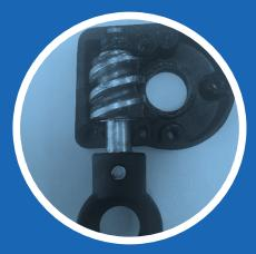
STEP 3: Turn the turbine component upside down and place back in it's position.
